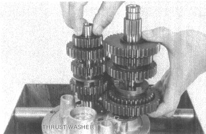
Press the gear assembly into position by lightly tapping the mainshaft with a soft hammer.
